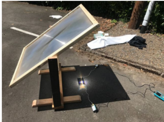
Figure B.2: Experimental set up for the characterization of the Fresnel lens. An aluminum block was placed at the focal point of the lens. One thermocouple was placed 10 cm away from the focal point (above) and another was placed near the focal point (below).
