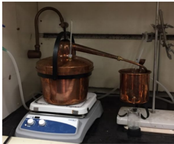
Figure A.4: Experimental setup for estimating energy required for a batch distillation. The hotplate was used to heat the still (left). Distillate travels from the still to the condenser (right).
